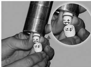
6. Connect the plug of the rotational arm and the socket of the stud;
