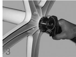
3. Get the screw across the piece of round iron, wind the screw into the bottom of the stud, then screw down it with a wrench in the direction of the hour hand;
